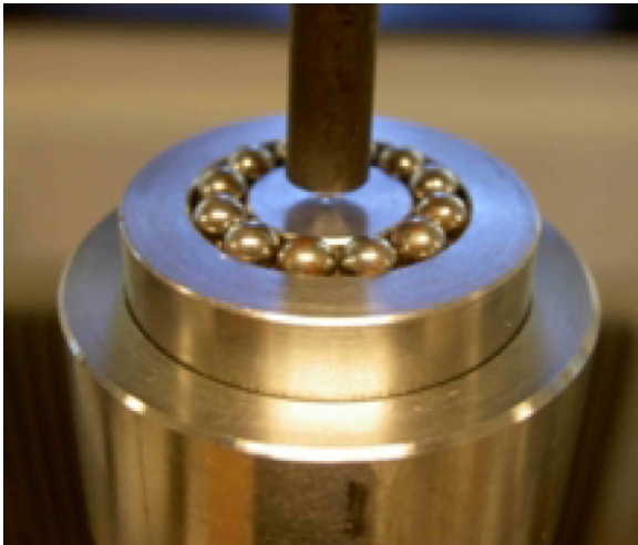
Fig. 1. Ring of supporting balls and piston for compression (no specimen).
